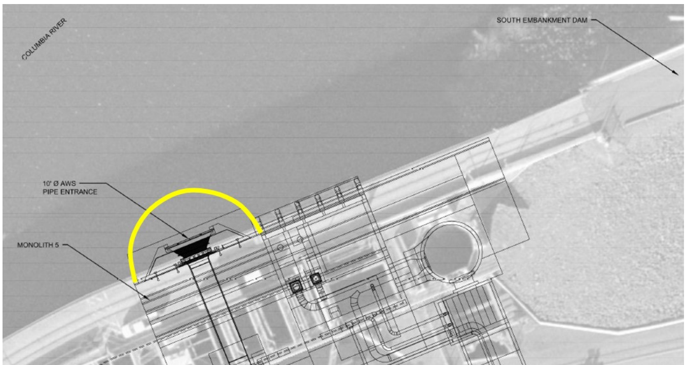
Plan view of existing entrance to AWSBS with triangular and semicircular floating boom or floating curtain
